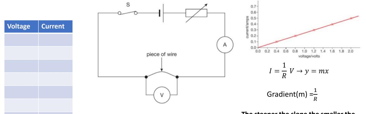
The steeper the slope the smaller the resistance
