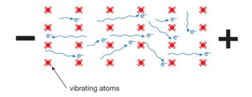
□ The resistance of a metal is higher at high temperatures.
