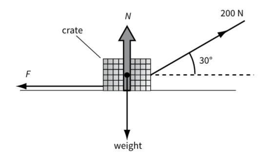
Calculate the work done on the crate by: i) the 200 N force. ii) the weight of the crate. iii) the normal contact force N. 2) A man pulls a box along horizontal ground using a rope. The force provided by the rope is 200 N, at an angle of 30° to the horizontal. Calculate the work done if the box moves 5.0 m along the ground.
