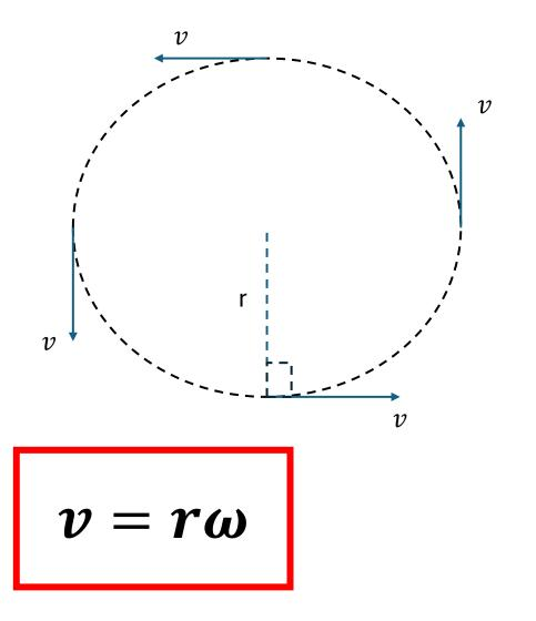
The linear velocity of the object at a point is called instantaneous velocity.
